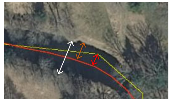
Figure 4-6: Normalizing Centerline Offset Red line is measured center, yellow is modeled. White arrow is bankfull-width, orange arrow is "bank-distance," red line is centerline offset.
