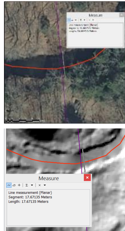
Figure 3-10: Manual Width Measurement Longer purple lines show field-measured cross-sections. Shorter white lines show manually estimated widths.
